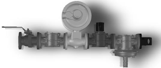
The gas filter protects the gas train and engine from particulate contaminants that may be present in the gas stream. The Gas Train is regulated to accept 1-5 psi gas pressure supply. The gas lock off solenoid is a 24V single stage solenoid, controlled by the PLC. The zero pressure regulator detects changes in engine vacuum through the mixer to maintain slightly below atmospheric pressure.
